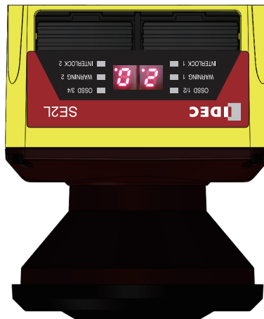
Figure 3-27 Example of upside-down configuration (The area number is 02.)
