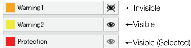
Figure 7-46 Switching between visible and invisible mode
