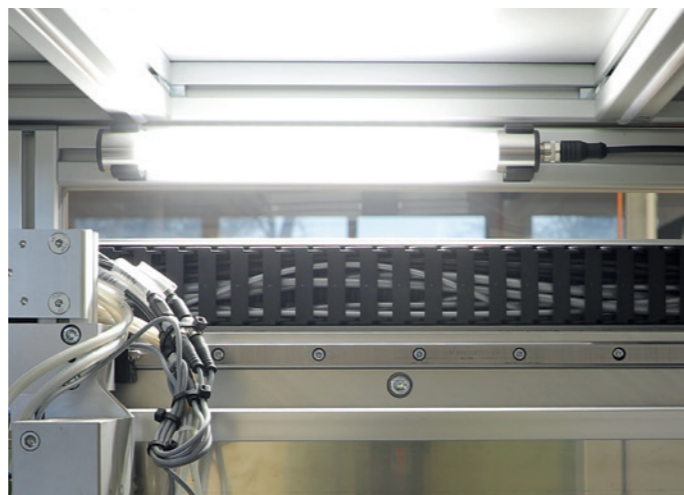
LED tube in polycarbonate
