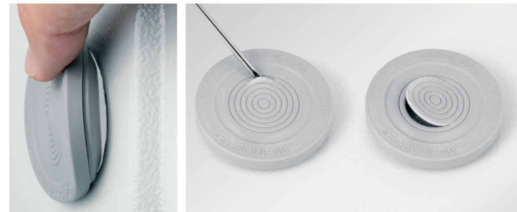
The single membrane rings are peeled off according to the diameter of the routed cable or hose. For this purpose, only a small hole between the rings needs to be pierced. Then the corresponding ring can be removed.
