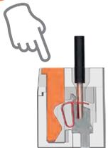
Push the actuator button to close the terminal.
