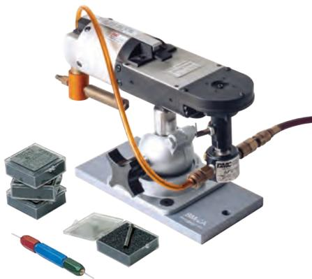
insertion tool - removal tools replacement tip
