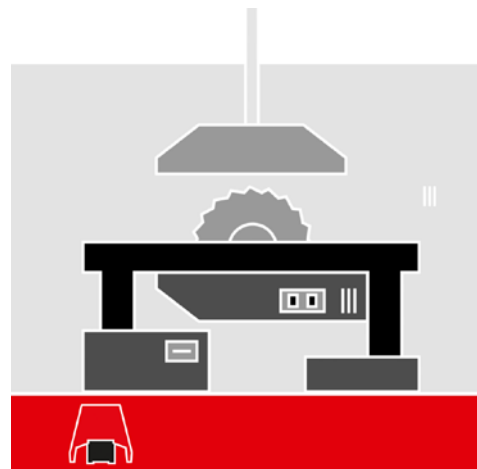
Foot switch with safety catch and manual release on a woodworking machine
