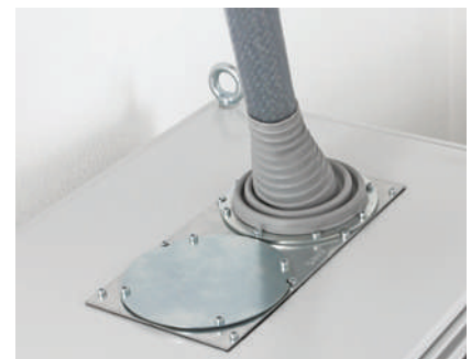
Routing of a rigid supply line through a closed enclosure roof via module plates. Cut-out size 314 x 144 mm.
